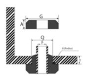
The two piece Mountings are an ideal product for both mobile & static applications for reducing vibration, allowing flexibility within a system and are used for reducing stresses on brackets etc. Using washers ensures a failsafe mounting system arrangement. A = Thickness Of Rubber Bush.
